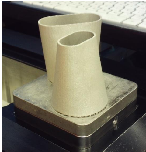
Figure 5.23 3D Printed Transition Couplings
