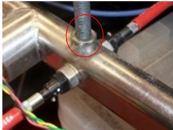
Figure 6.7 Access point for lens purging during testing
