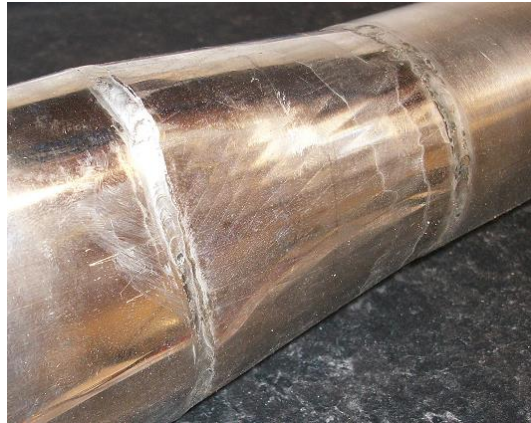
Figure 5.27 Welded Transition Couplings
