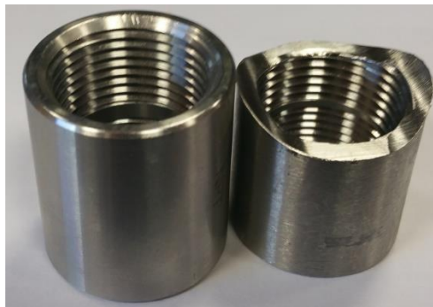
Figure 5.26 Modified NPT Coupling
