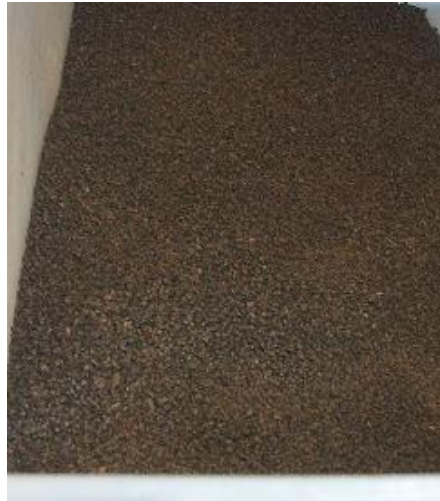
Figure 5.13 Granulated blend of 50% Coffee, 50% Sugar in baking tray after removal from oven
