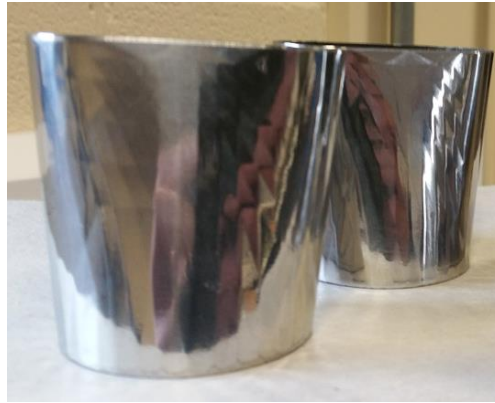
Figure 5.24 transition Pieces After Polishing process
