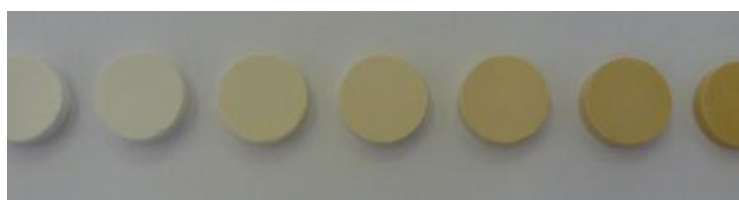
Figure 3.4 Pharmaceutical tableting process and the effect of a deviation in ingredient concentration on the colour of the product (Colour measurement of tablets in pharmaceutical production | Micro-Epsilon Measurement, 2017)
