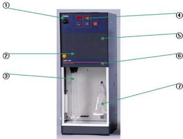
1. Turn on/off 2. Steam generator 3. Kieldahl tube 4. Conical flask with boric acid 5. Pumps 6. Cooling water sensor 7. Flask with boric acid Figure 1.29: 2100Kjeltec Distillation Unit. Source: (Busan, 2006).
