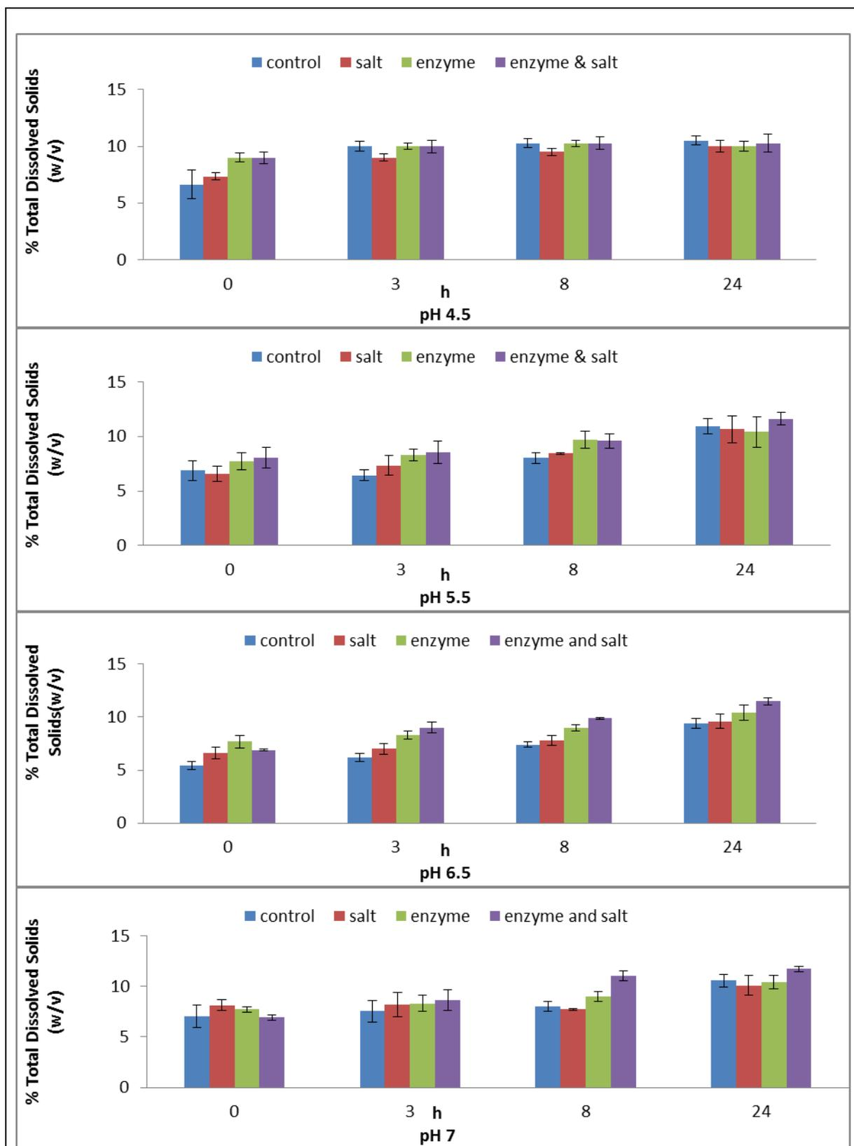
Figure 3.4 Total dissolved solids (%w/v) in extracellular medium during the induced autolysis of SDYK in the presence and absence of salt and enzyme papain, at 50°C and at different initial pH values. The values presented are the means of four replicate trials.
