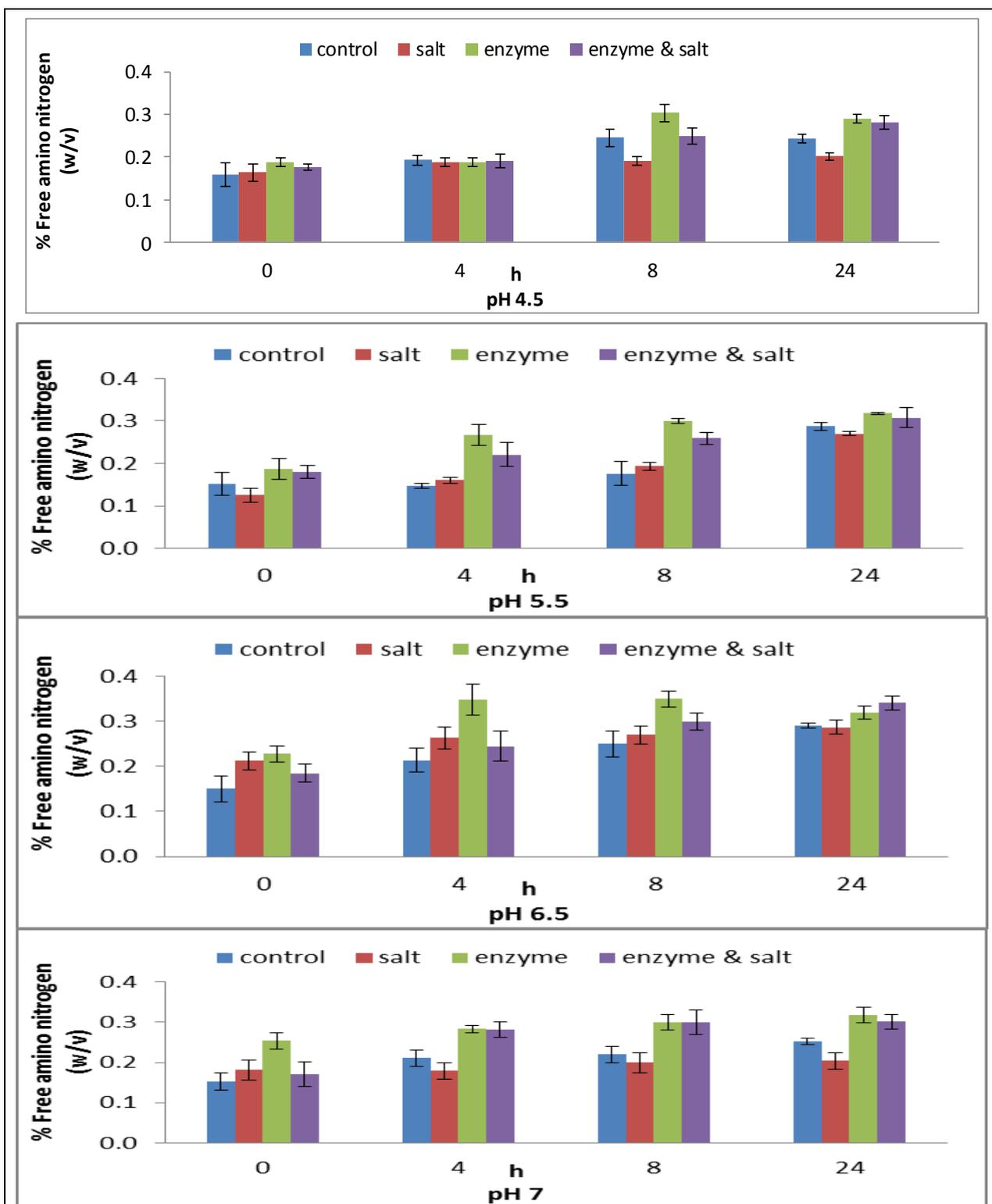
Figure 3.1 Free amino nitrogen released during autolysis of SDYK at various initial pH values, in the presence and absence of salt and enzyme papain. The values presented are the means of four replicate trials.
