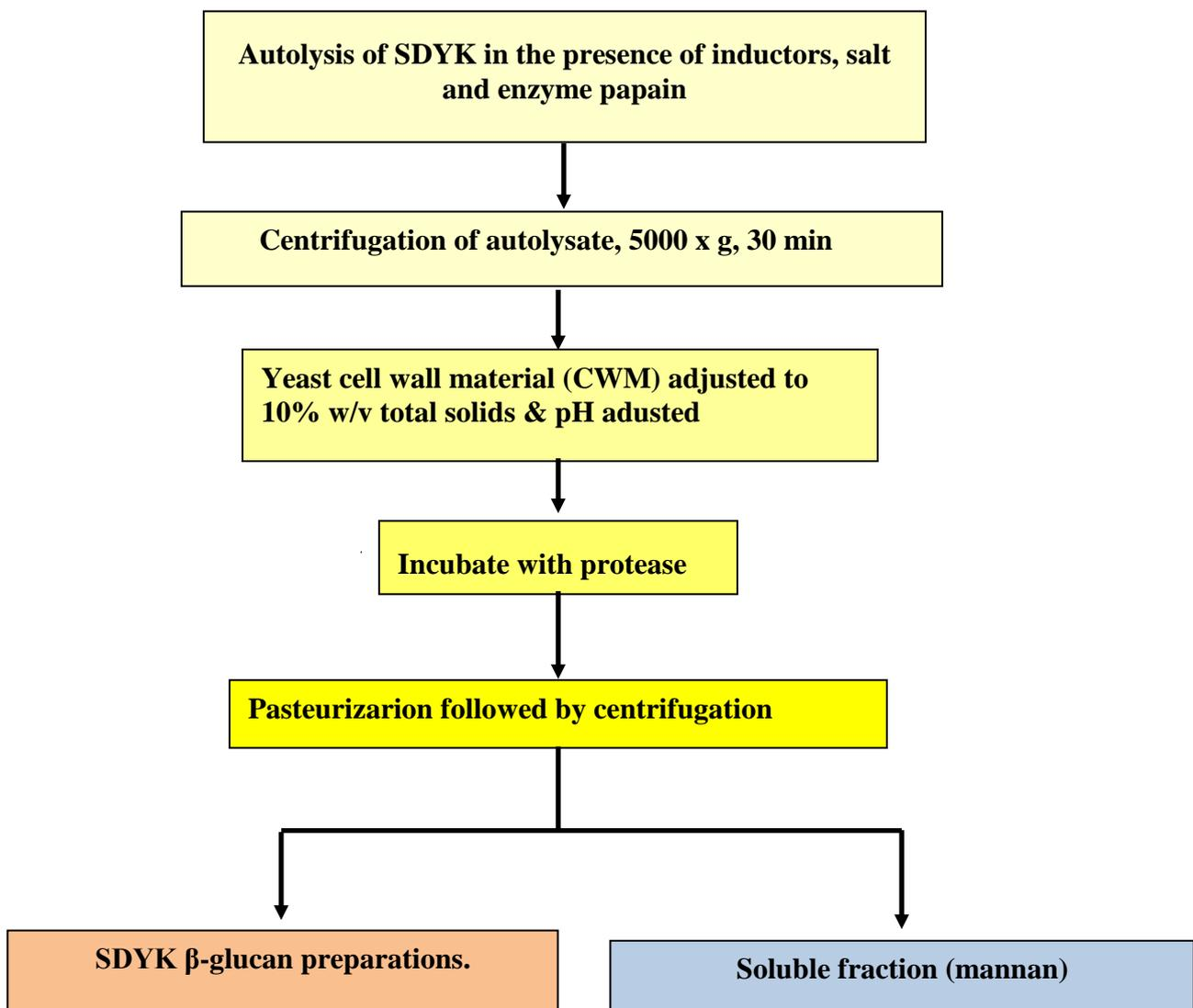
Figure 3.9 Flow diagram of a natural enzymatic process for isolation of yeast cell wall polysaccharides from SDYK.
