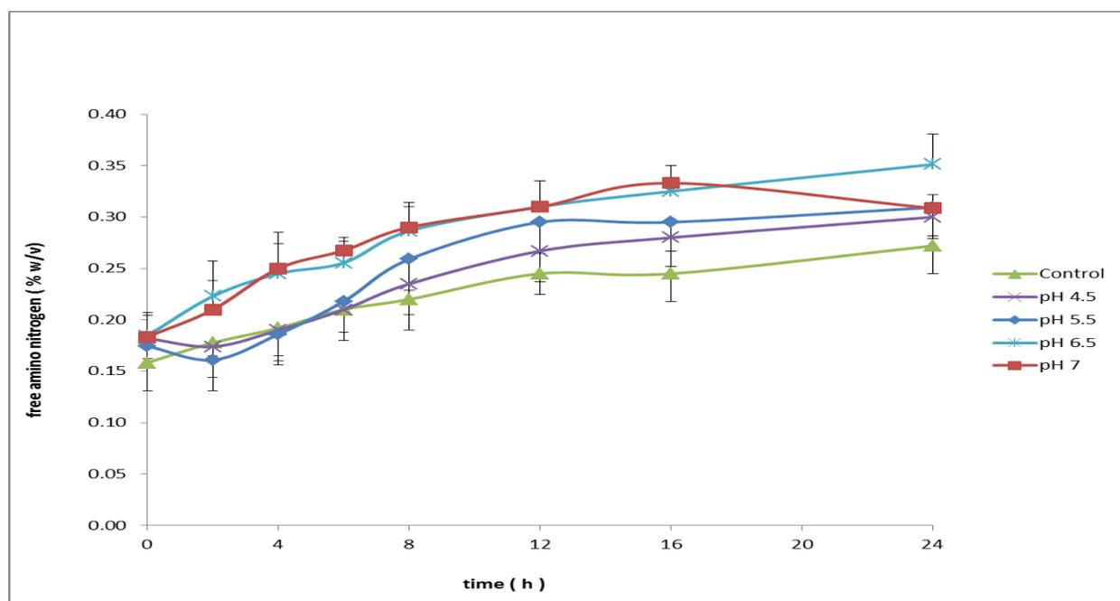
**Figure 3.2** Time course of the % free amino nitrogen released into extracellular medium during the autolysis of SDYK at 50°C, at different initial pH values in the presence of salt and papain. The values presented are the means of four replicate trials.
