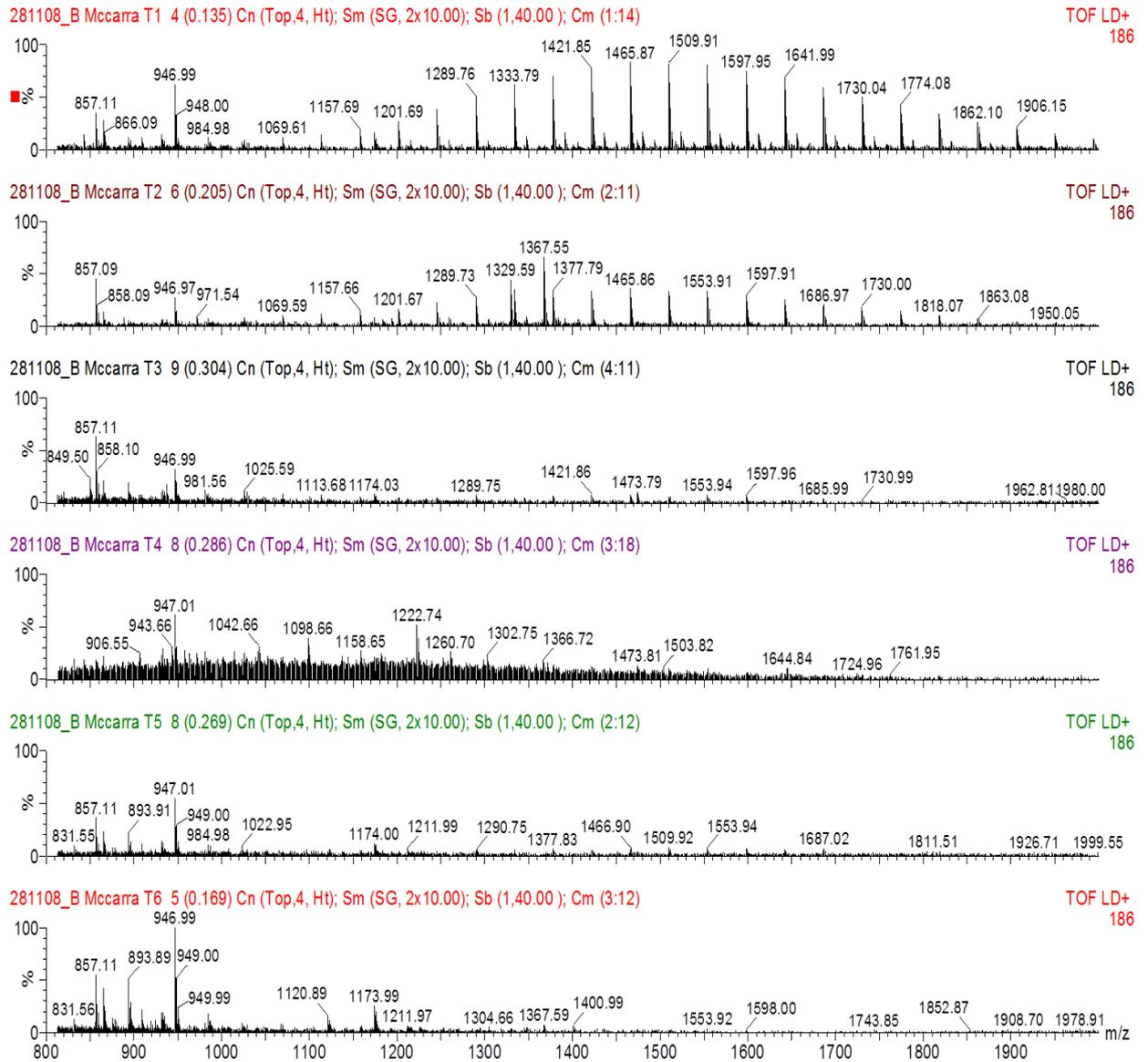
**Figure 4.16 LC Mass-Spec of SEC fractions (1000 Da) of T1 – T6 yeast extracts (SDYK) derived from different autolysis conditions.**
