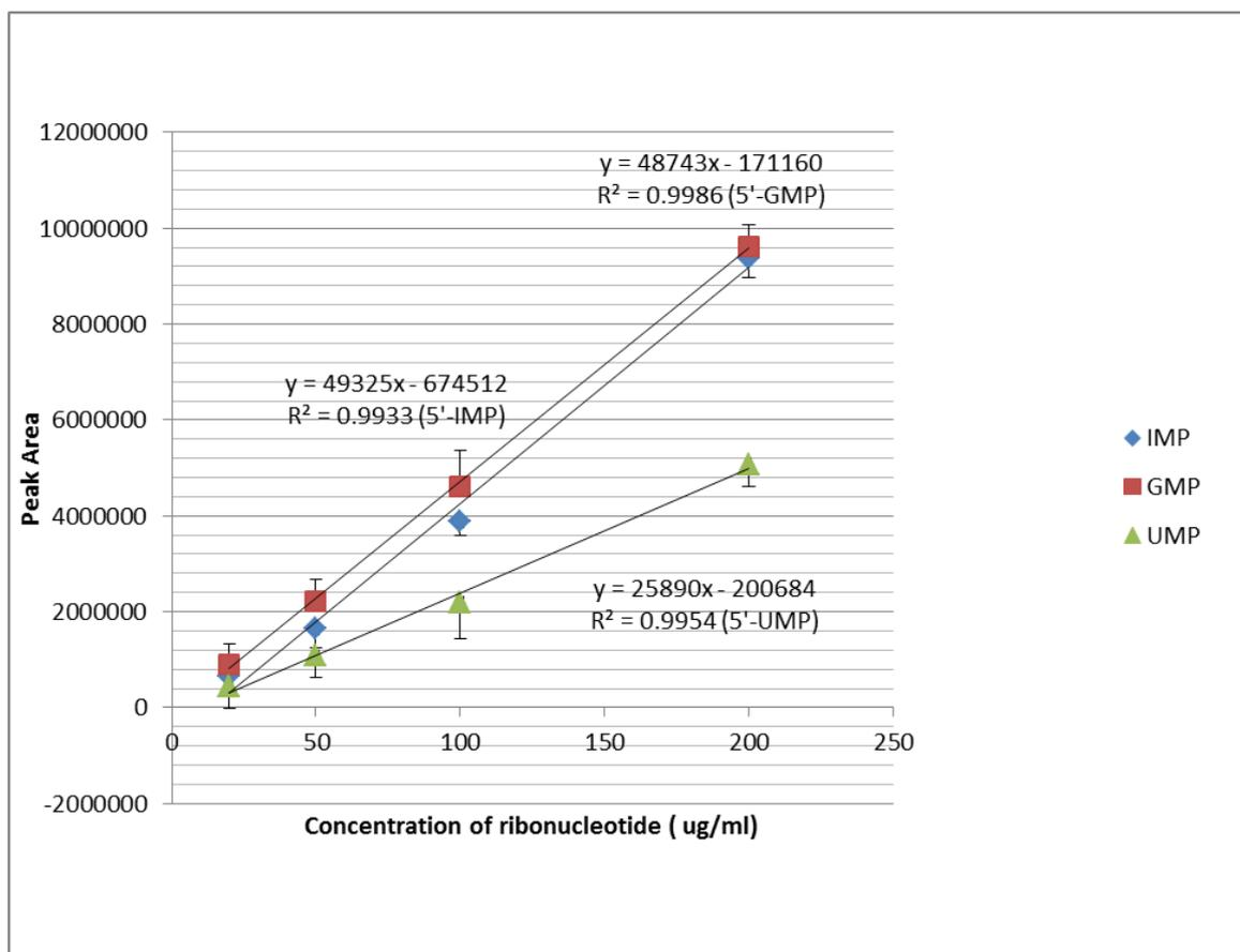
Figure 4.1 Standard curves for measurement of ribonucleotides using HPLC reversed phase chromatography.
