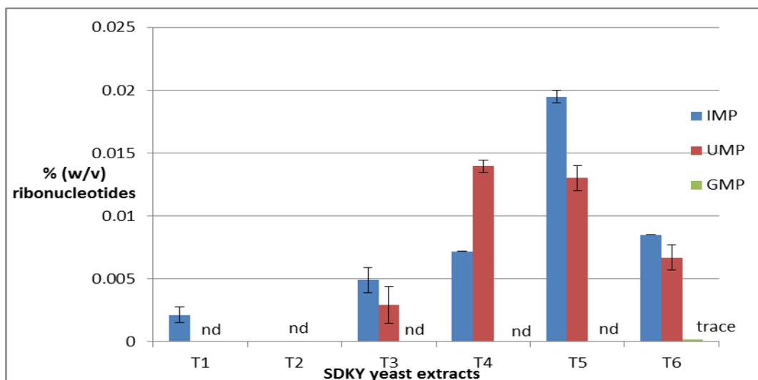
**Figure 4.9** Concentration of 5'ribonucleotides (%w/v) obtained in yeast extracts produced from induced autolysis of SDYK (nd = not detected).
