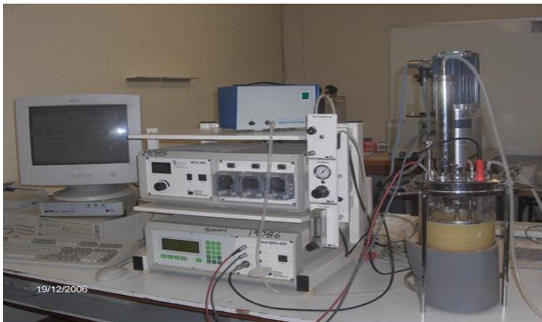
**Figure 1.1 Study of yeast autolysis during the course of this work using a five litre automated bioreactor system.**
