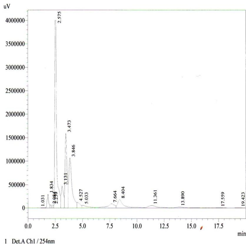
**Figure 4.10** Reversed phase HPLC chromatogram of yeast extract T4 indicating the presence of 5' IMP with a retention time of 11.36 min.
