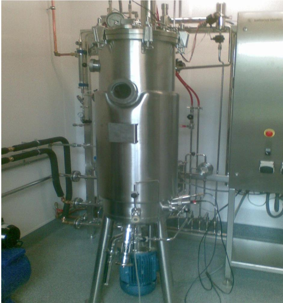
**Figure 1.16 The custom-engineered approach for a 100 litre bioreactor or fermentor system together with on-line sensors, touch-screen technology and advanced process control software. (Commissioned at Shannon Applied Biotechnology Centre, May, 2012).**
