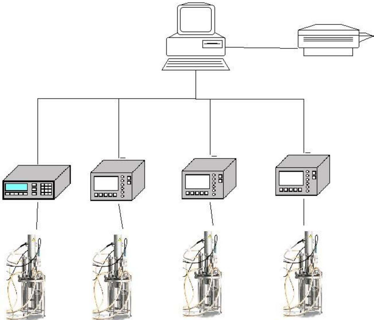
**Figure 1.14 Multiple bioprocesses can be controlled automatically from a single computer.**
