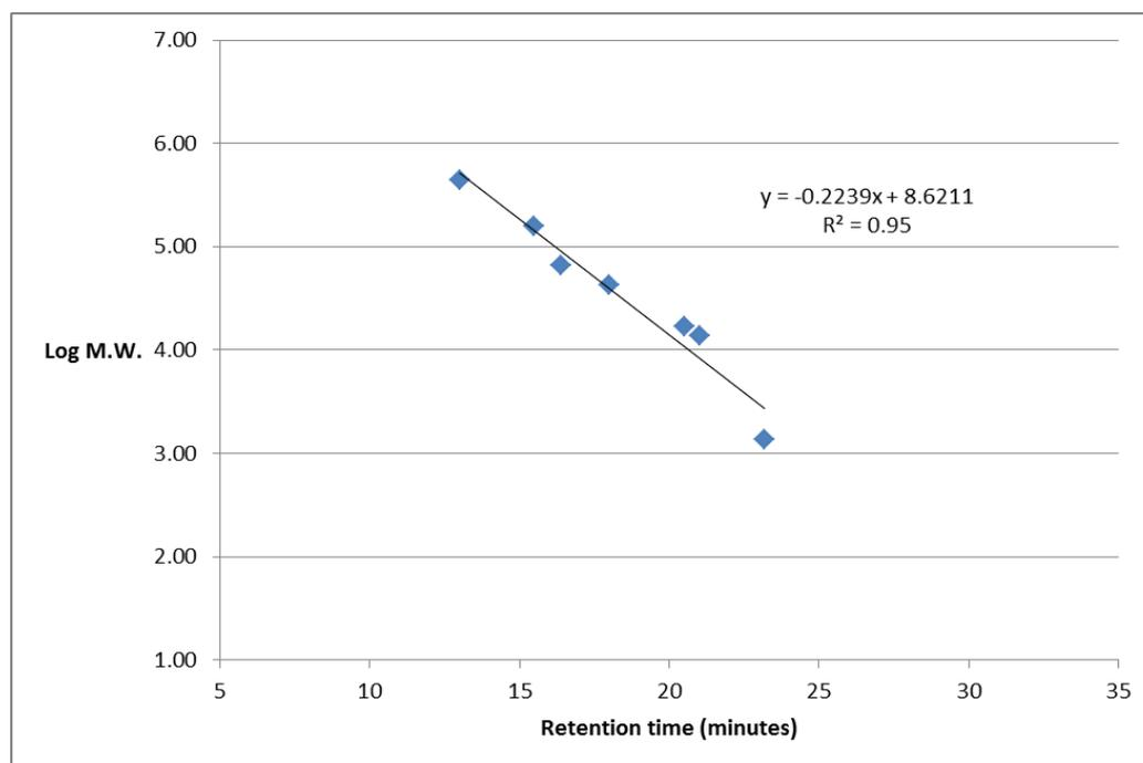
**Figure 4.2 Calibration curve showing relationship between molecular weight of protein standards (Da) and retention time on a Waters Protein-Pak HPLC size exclusion column.**
