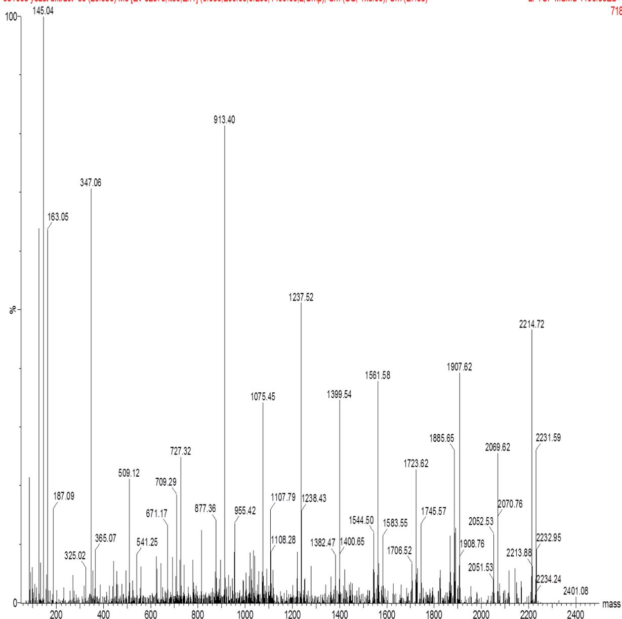
**Figure 4.15** Fragment ion spectrum (product ion spectrum) from the intact ion which was seen at mass 2209 (1105++) on the intact spectrum in Figure 4.14
