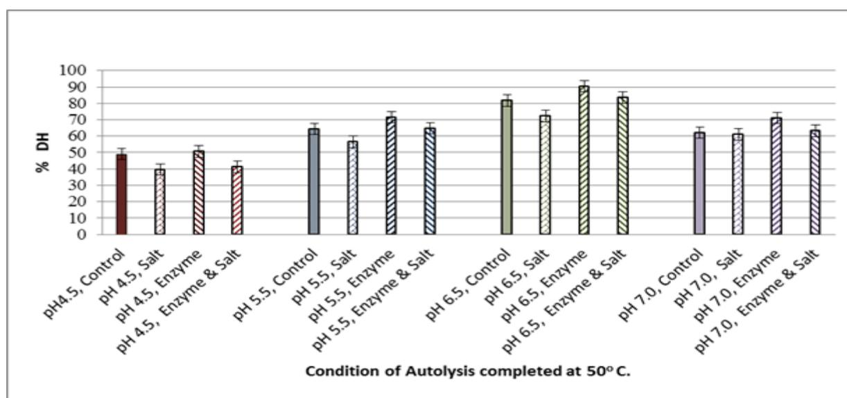
Figure 3.3 Overview of % degree of hydrolysis (% DH) of in extracellular medium after 24 h of induced autolysis of SDKY at 50°C, at different initial pH values in the presence and absence of salt and enzyme papain. The values presented are the means of three replicate trials.
