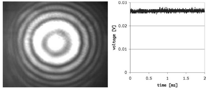
Fig. 3. Left: Fringes produced by interfering two mutually coupled, 1.3 m separated quantum dot lasers. The phase coherence between the two lasers is evident in the high visibility of the fringes generated. Right: oscilloscope trace with 1.5 GHz bandwidth of a 1 mm long QD-FP laser coupled to 600  $\mu\text{m}$  long QD-FP laser, 1.3 m distant.
