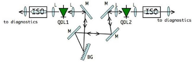
Fig. 1. Experimental arrangement for investigating the dynamics of bi-directionally coupled QD-FP lasers, QDL1 and QDL2. The blazed grating BG is included to ensure single mode operation. Optical isolators (ISO) prevent external reflections from perturbing the system.
