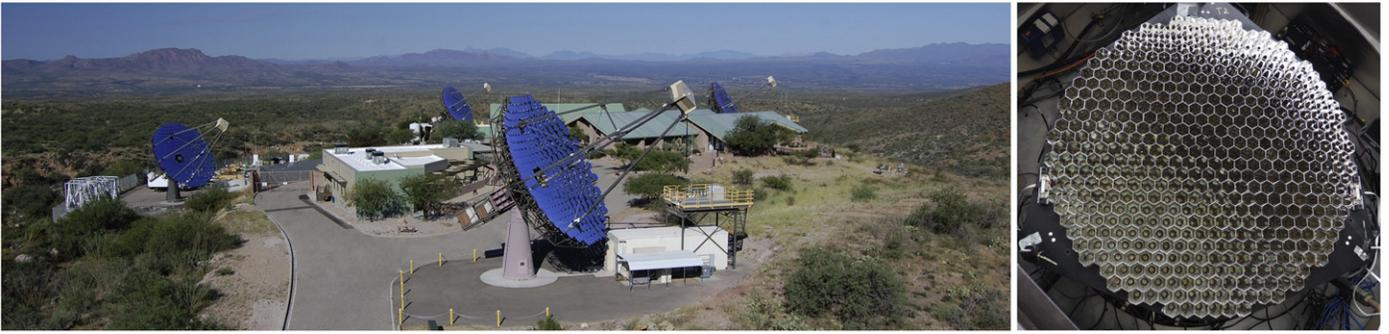
**Figure 1.** The VERITAS array in Arizona (left) and the PMT camera of a single telescope (right). The camera covers a total field of view of diameter  $3^{\circ}.5$ . The hexagonal reflective light cones reduce the dead space between the circular PMTs.
