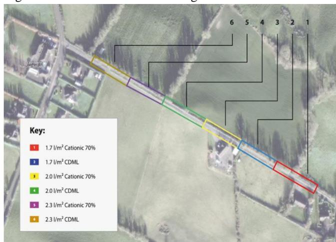
Figure 2: Aerial view of site trial including rates of spread of emulsion
