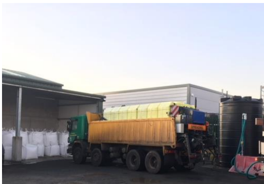
Figure 4 Hired Boschung 11,550 Litre Capacity Liquid Hopper Mounted on Offaly County Council Owned 32 Tonne Tipper
