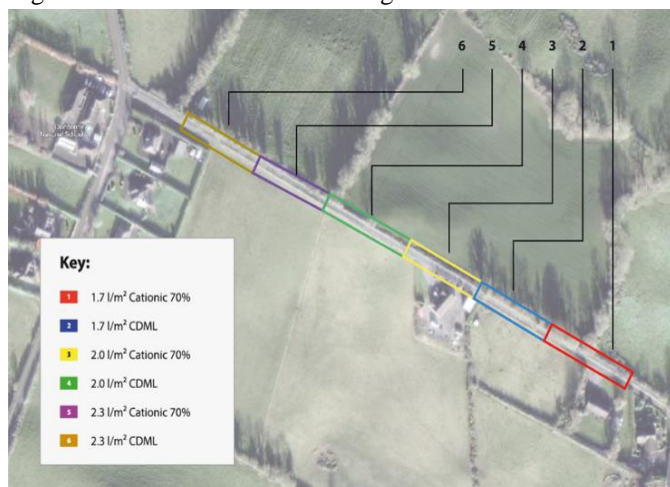
Figure 2: Aerial view of site trial including rates of spread of emulsion
