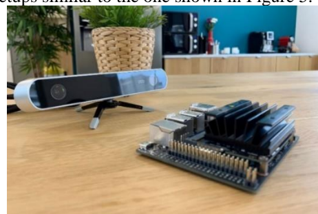
Figure 5 ZED Stereo Camera and Jetson Nano microcomputer.
