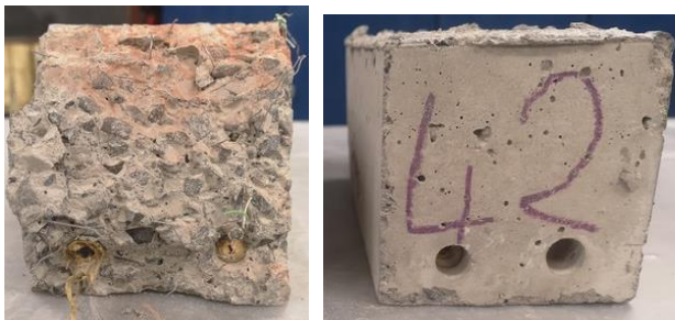
Figure 13. (a) A snapped pair of bamboo culms and (b) with debonding, the ends of the bamboo culms retract into the concrete upon flexural failure.
