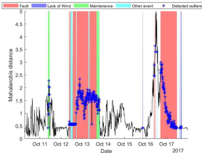
Figure 5. Mahalanobis distance for a 2-channel signal (power and wind speed) between the 10<sup>th</sup> and 22<sup>nd</sup> of October. Coloured areas show time periods with notable events for this turbine.
