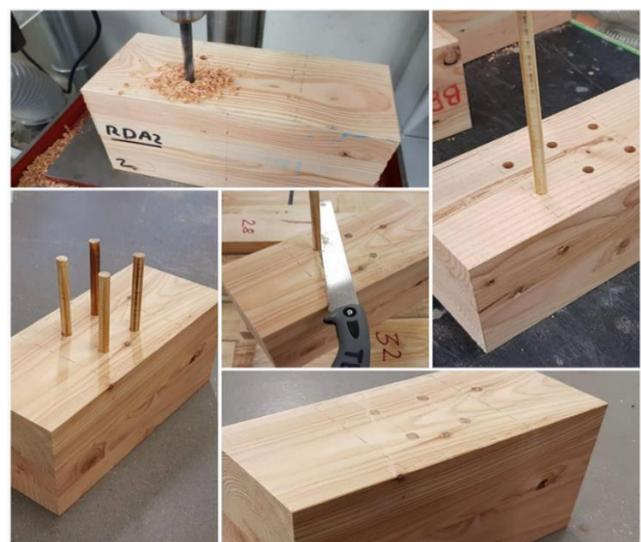
Figure 5.2 Specimen preparation
