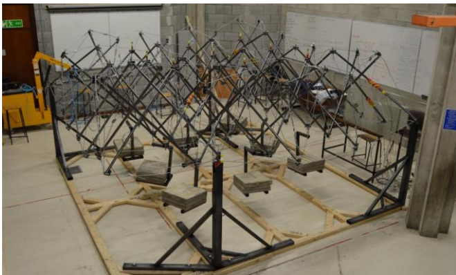
Figure 9. Grid test layout with structure partially loaded (increment 4 of 6)
