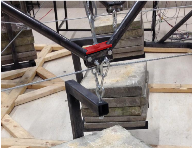
Figure 5. Inner node fixing plate (highlighted in red)
