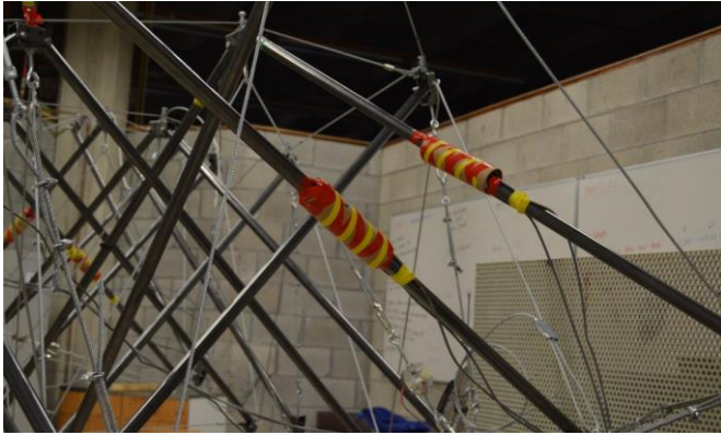
Figure 8. Instrumented compression struts with projective coverings over strain gauges
