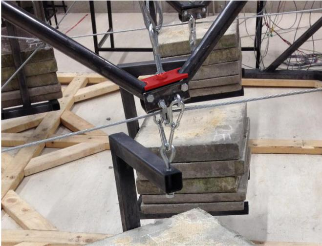
Figure 5. Inner node fixing plate (highlighted in red)
