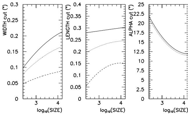
FIG. 1.—Upper (solid line) and lower (dashed line) “extended cuts” on the image parameters WIDTH, LENGTH, and ALPHA as a function of  $\log_{10}(\text{SIZE})$  with tolerance  $t = 2.0$ . These cuts minimize systematic errors stemming from the simulations. The dotted lines show the upper cuts for maximum significance above 2.5 TeV (optimized on Crab Nebula data; see § 3.7).
