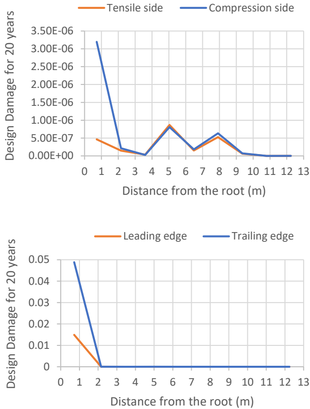
Figure 11. Design damage for 20 years along the blade
