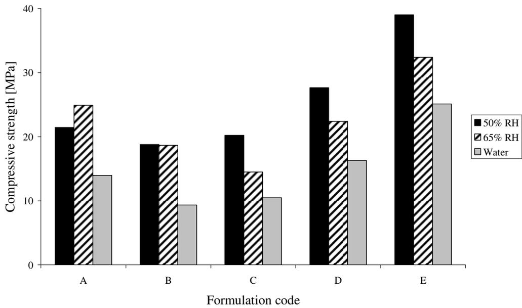
Figure 3. Stability of mortar prisms using calcium-sulfate based cements, when stored underwater.
