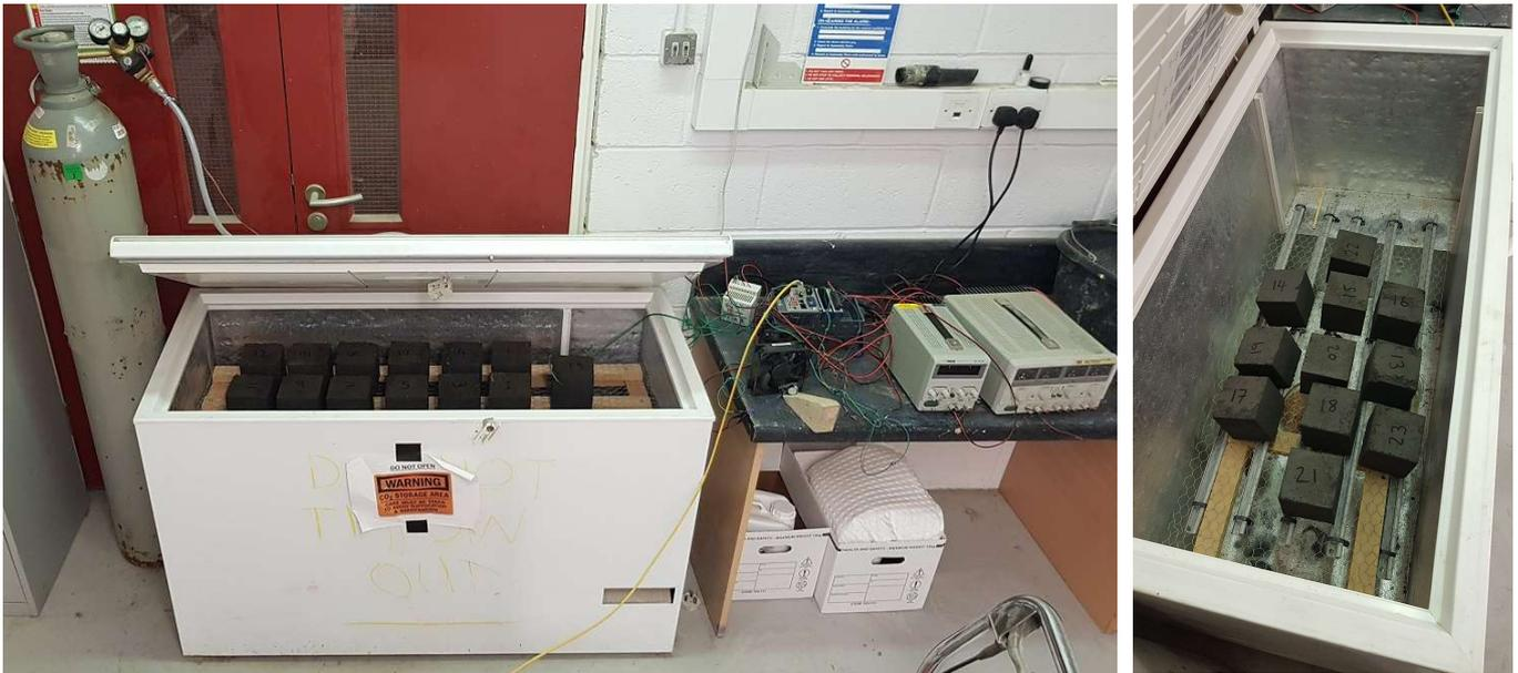
Figure 1. Accelerated carbonation curing chamber
