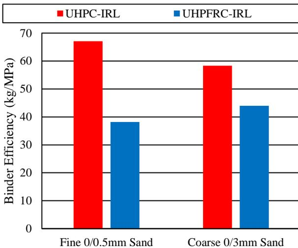
Figure 6. Binder efficiency of the mixes in tension
