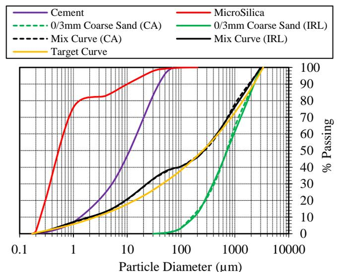
Figure 3. Mix target curve (q=0.23) and the resulting integral grading curve of the composed UHPC-0/3 coarse sand mixes.
