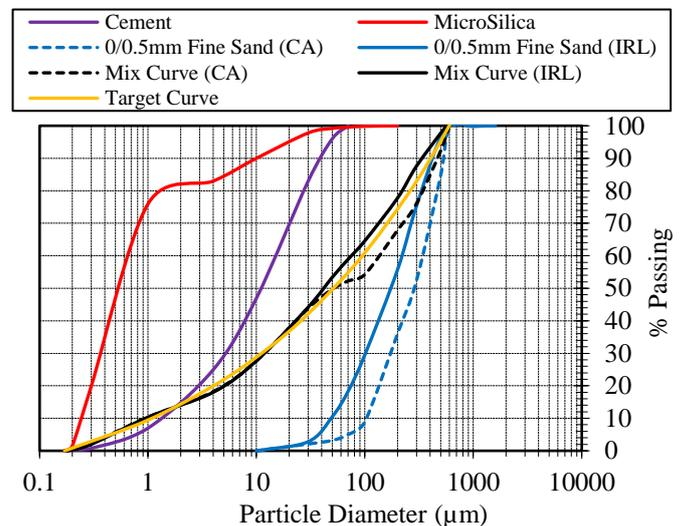
Figure 2. Mix target curve (q=0.22) and the resulting integral grading curve of the composed UHPC-0/0.5 fine sand mixes.
