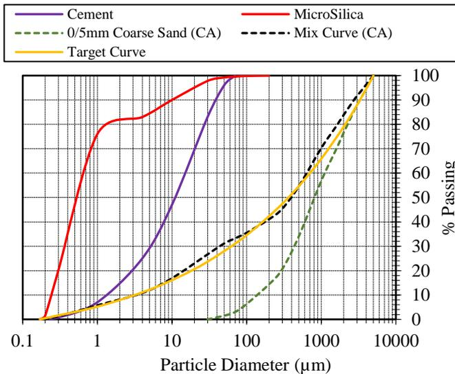
Figure 4. Mix target curve ( $q=0.23$ ) and the resulting integral grading curve of the composed UHPC-0/5 coarser sand Canadian mix.
