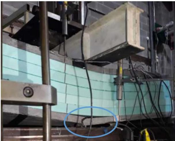
Figure 10. Image of the unconnected sandwich panel close to failure
