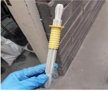
Figure 1. 200mm long FRP shear connector
