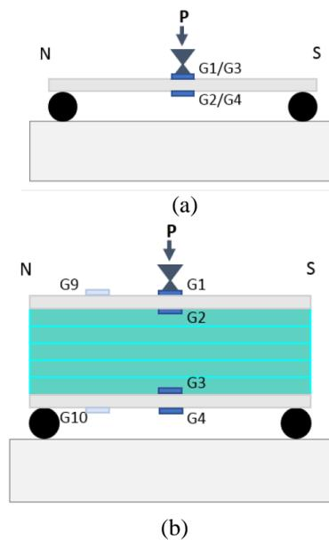
Figure 2(a) Flexural test arrangement for a single wythe and (b) typical sandwich panel with clear span 850mm
