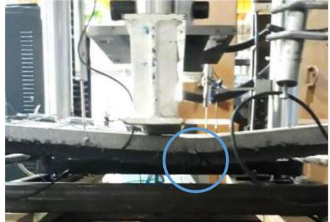
Figure 8. Fully developed crack under peak load for ribbed single wythe
