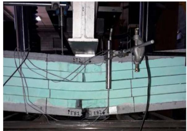
Figure 12. Image of the shear connected sandwich panel close to failure
