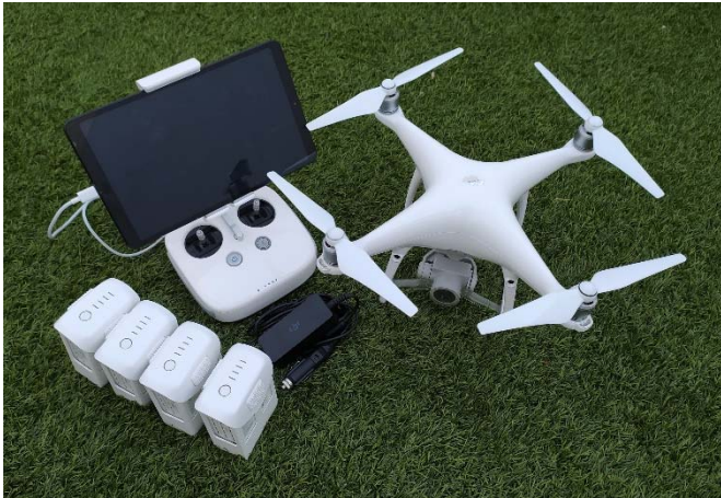
Figure 4. DJI Phantom 4 Advanced used for the traffic monitoring
