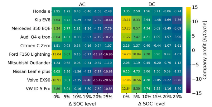
Fig. A.6. Analysis of the company profit per full cycle of the 10 EV models under different \Delta SOC (0 to 25%) for AC and DC charging scenarios.
