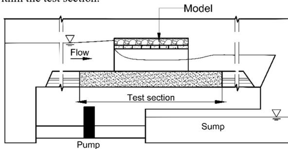
Figure 1. Schematic of the flume and test setup (not to scale) and instrumentation not shown
