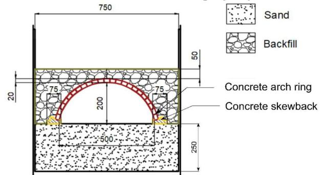
Figure 2. Cross-sectional schematic of the single span FlexiArch bridge model (dimensions in millimetres)
