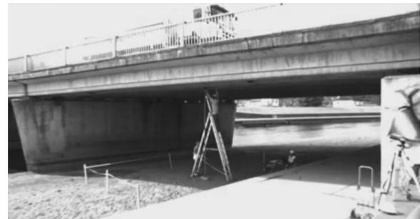
Figure 4. Monitoring installation on bridge as truck passes over midspan during Loaded Swipe 1
