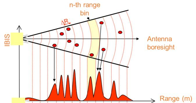
Figure 3. IBIS-FS Method of Measurement - Range Resolution
