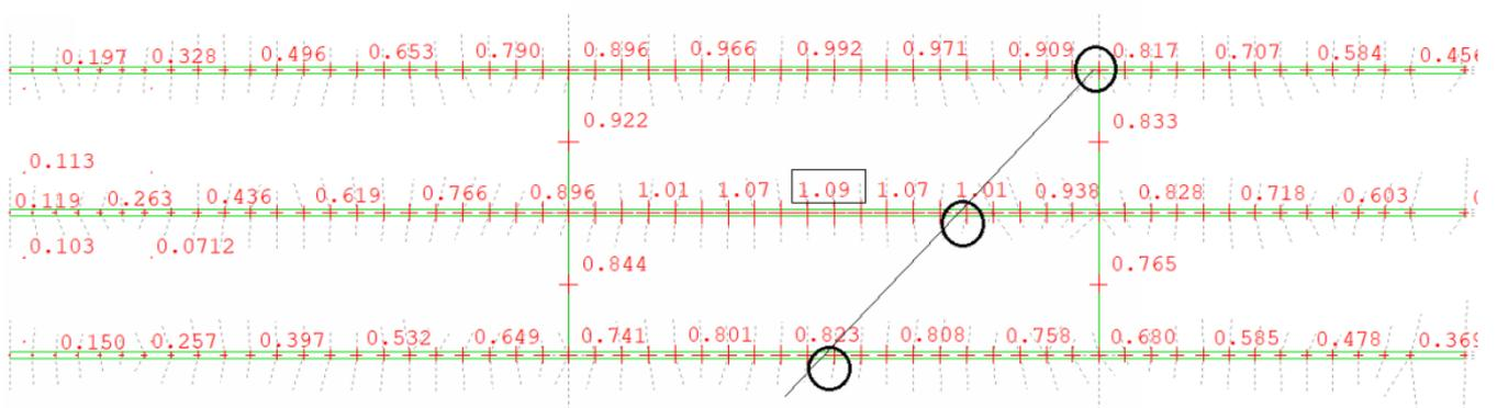
Figure 11. FEM obtained displacements with adjusted axle load
