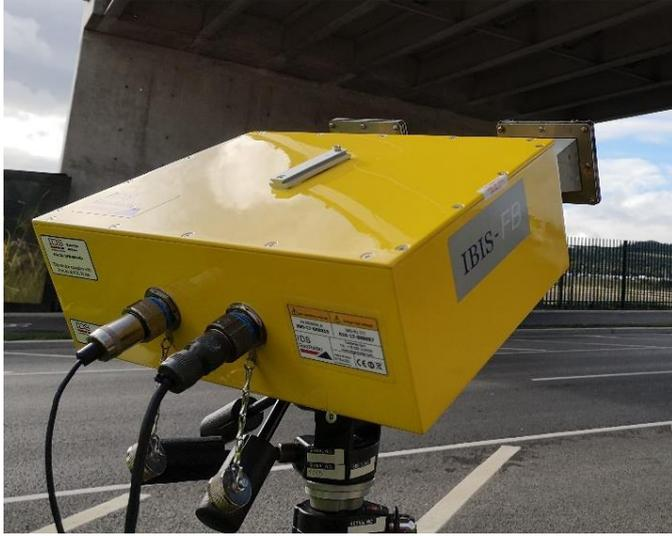
Figure 2. IDS GeoRadar IBIS-FS Interferometric Radar
