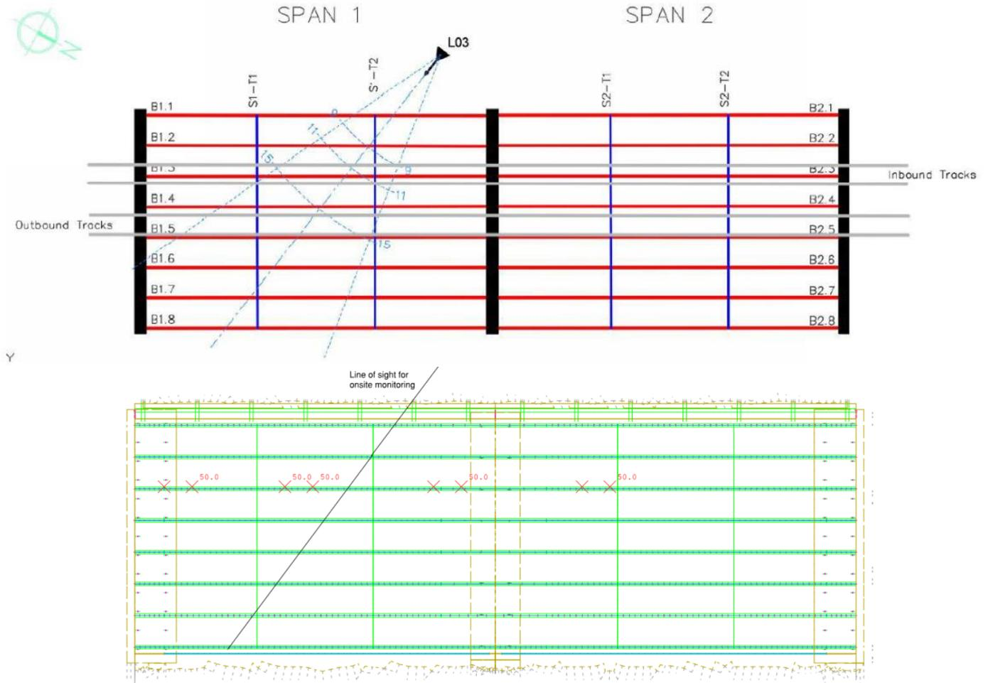
Figure 10. Bridge structural member naming convention, instrument set up location, radar line of sight and range bins for set up (above) and superimposed in the FEM model (below)
