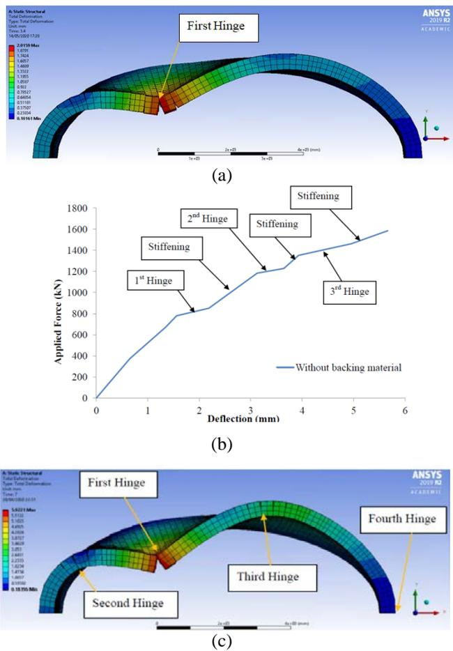
Figure 13: Model of Bridge No.1 without structural backing indicating (a) formation of first hinge, (b) load-deflection curve indicating hinge formation, and (c) location of all hinges.
