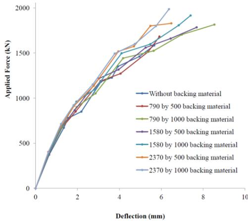
Figure 7: Load-deflection response for Bridge No. 1.
