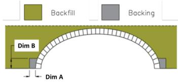
Figure 6: Location of concrete structural backing
