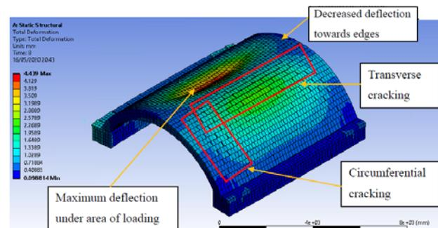
Figure 12: Deformation behaviour of Bridge No.2 without backing (only arch is shown for clarity).
