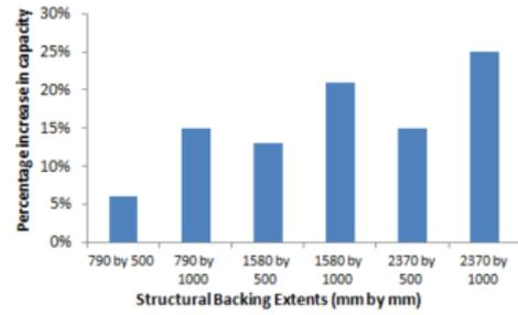
Figure 9: Percentage increase in capacity for Bridge No. 1.
