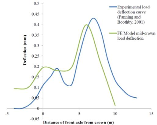
Figure 5: Comparison of experimental [8] and FE model deflections under moving vehicle load.
