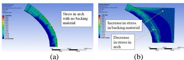
Figure 16: von-Mises stress distribution in arch of Bridge No. 1 in (a) without backing material, and (b) with 2370mm by 1000mm backing material.
