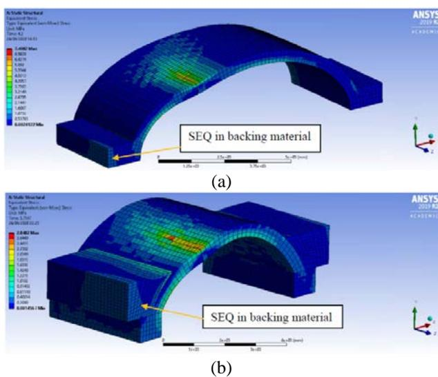
Figure 15: Distribution of SEQ in models with structural backing for (a) 790mm by 1000mm backing in Bridge No.1, and (b) 1130mm by 1000mm backing in Bridge No.2
