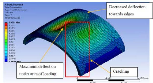
Figure 11: Deformation behaviour of Bridge No.1 without backing (only arch is shown for clarity).
