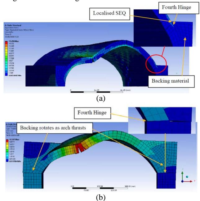
Figure 14: Location of fourth hinge in models with structural backing for (a) Bridge No.1, and (b) Bridge No.2
