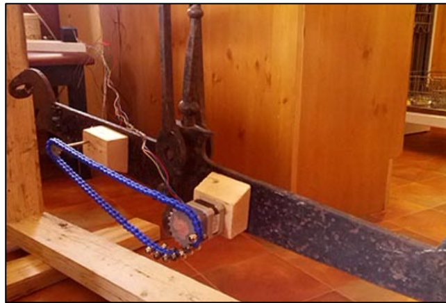
Figure 4.13 A stepper motor was placed on the rear of the balance. The stepper motor moved a chain that had weights attached to it, causing it to move between balanced and imbalanced positions.
