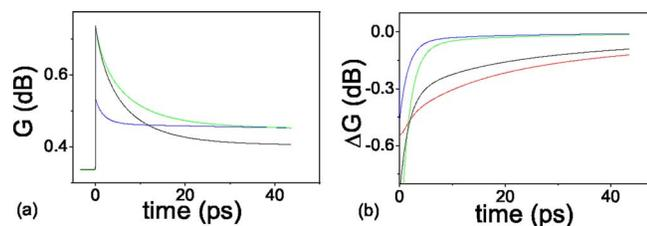
FIG. 3. (Color online) Simulated recovery of absorption (a) and gain (b). (Blue) ES pump GS probe, (green) GS pump GS probe, (black) ES pump ES probe, and (red) GS pump ES probe. Parameters were  $J=0.01$  (absorption), 1 (gain),  $\gamma_0=1$ ,  $\gamma_1=1$ ,  $\gamma_2=10$ ,  $\gamma_h=2$ ,  $\gamma_s=0.01$ ,  $\epsilon_1=0.01$ , and  $\epsilon_2=0.1$ .
