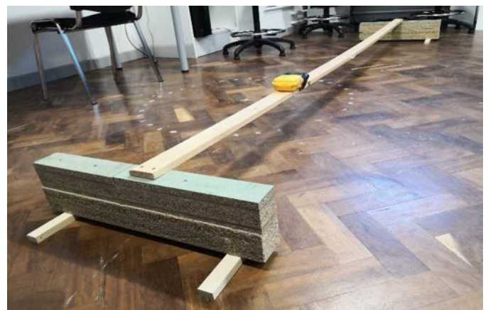
Figure 6: Simply-supported beam used for dynamic tests with data logger at the quarter-span point.
