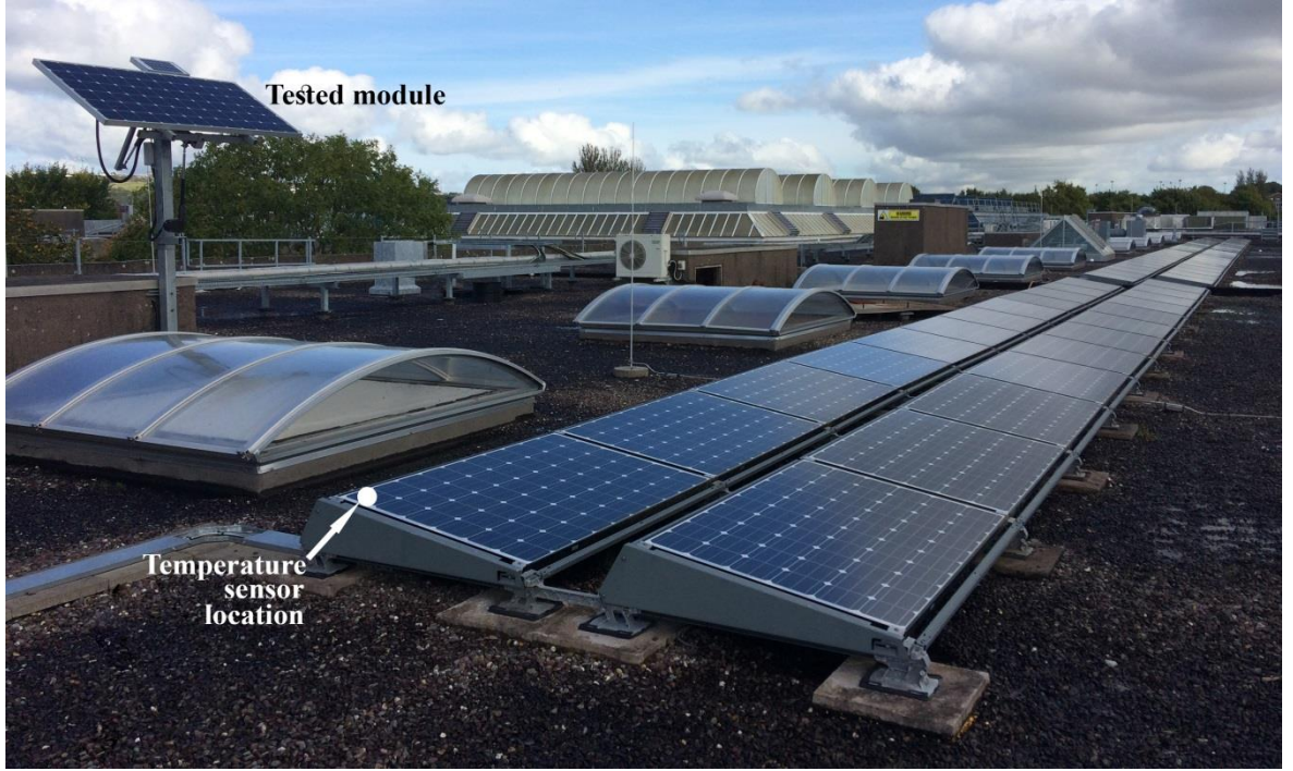
Figure 3.39: Temperature sensor location for the experiment
