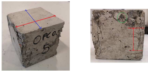
Figure 9 (a) Calibrating the concrete cube (b) Crack measurements
