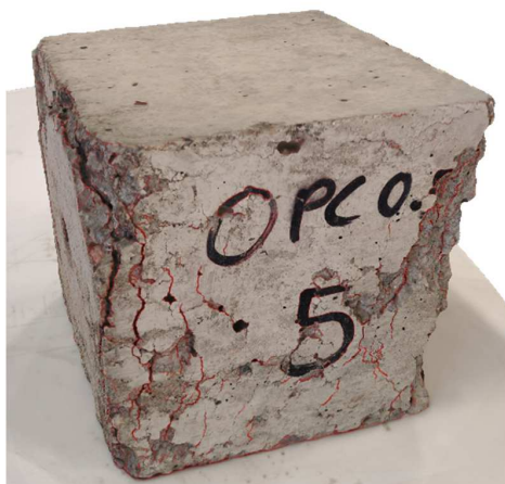
Figure 6. Concrete cube 3D model with crack locations marked on the model
